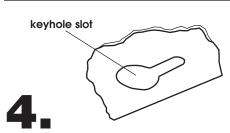
Lift range hood into final position and center. Mark on underside of cabinet the location for the four keyhole mounting slots. Set range hood aside on a protected
